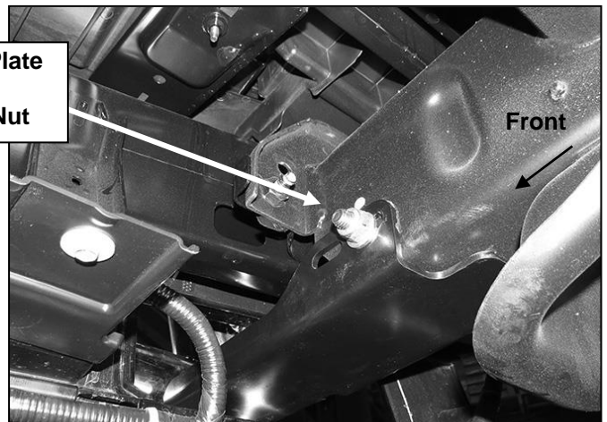
(Fig 11) Passenger Bracket installed in "forward" position to move Bull Bar away from bumper
