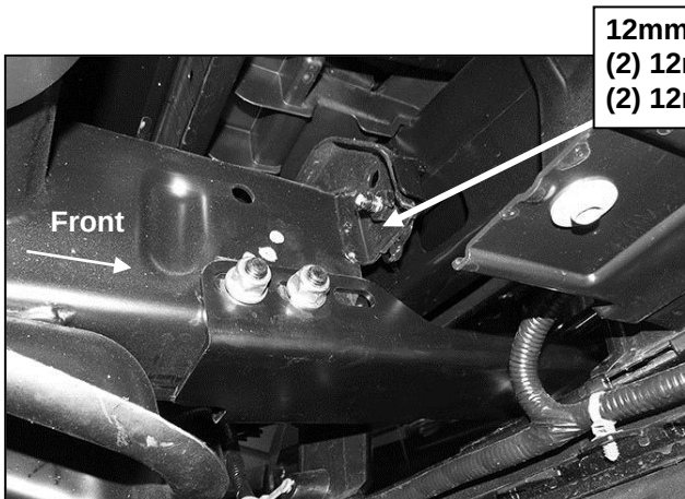
(Fig 6B) Note Bracket installed in "forward" position to move Bull Bar away from bumper
