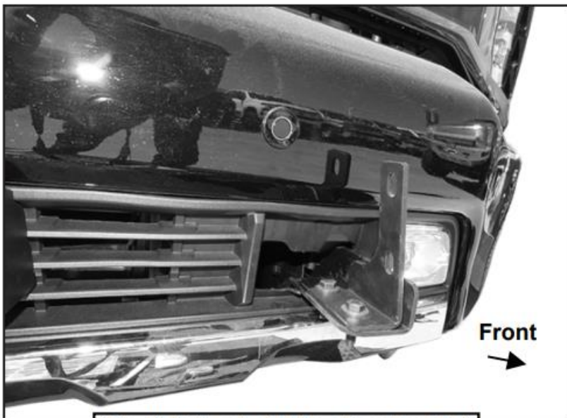
(Fig 7) Driver/Left Mounting Bracket attached to the Frame Bracket
