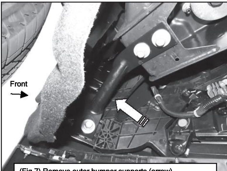
(Fig 7) Remove outer bumper supports (arrow)
