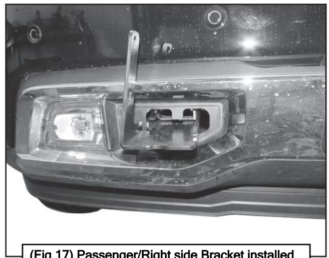
(Fig 17) Passenger/Right side Bracket installed
