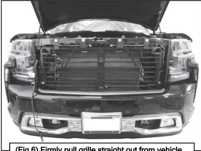
(Fig 6) Firmly pull grille straight out from vehicle
