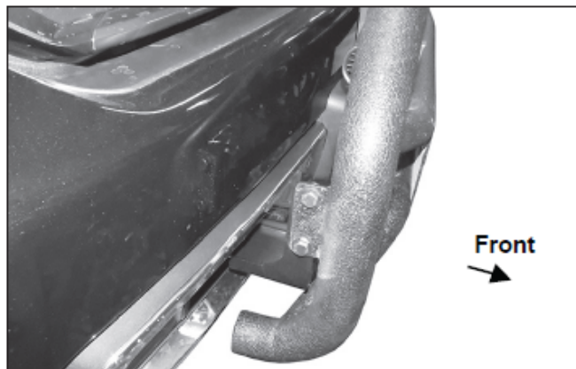
(Fig 19) Passenger/Right side complete installation
