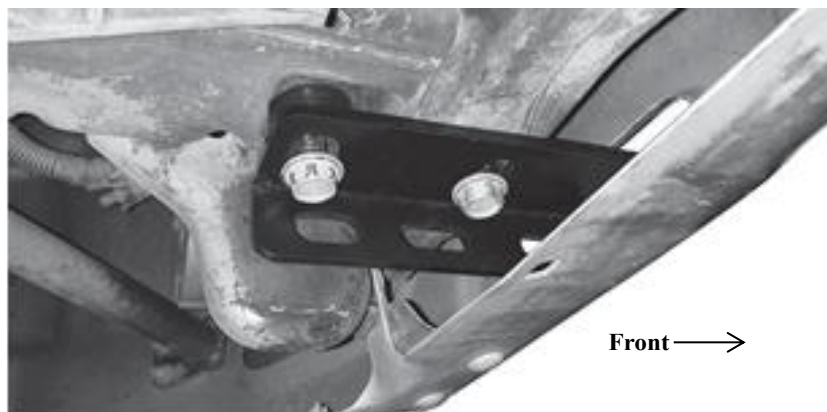
(Fig 5) Attach driver/left Frame Bracket to frame
