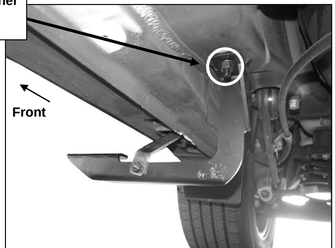
(Fig 10) Passenger side rear bracket installed
