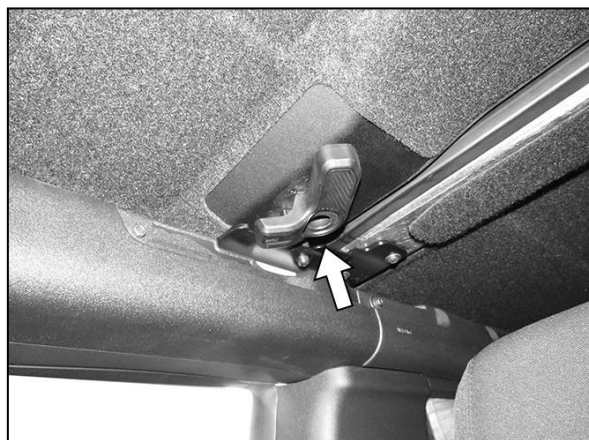
(Fig 18) If necessary, loosen screw 2-3 turns to adjust and fasten latch (arrow)
