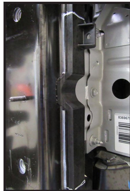
13. Using a reciprocating saw, trim the frame as shown. Do this on both sides of the vehicle.
