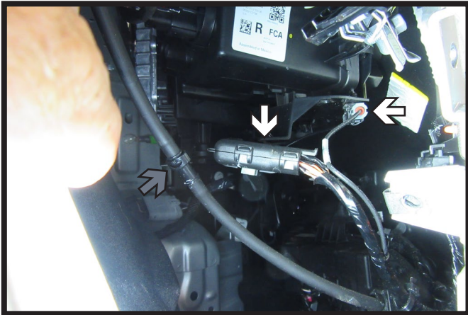
10. Unplug two (2) electrical connections (white) on the passenger side of the vehicle. Then disconnect windshield washer fluid line (gray).
