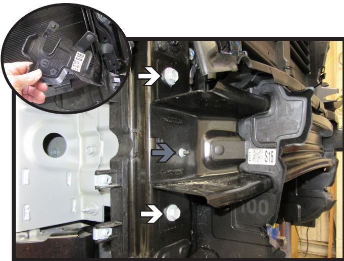
12. Using a 16MM socket, remove the two (2) bolts (white) from the bumper. Then using a 10MM socket, remove the one (1) nut (gray). Do this on both sides of the vehicle. Remove bumper and set aside. It will not be reinstalled later. As the bumper is removed, remove two (2) push pins from shroud piece around bumper (inset). Remove shroud piece.
