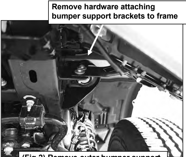
(Fig 2) Remove outer bumper support
