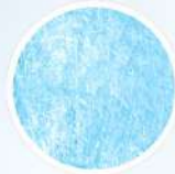
Magnified at 300x HEPA Media Three Layers
