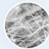
Magnified at 300x Non-HEPA Media Two Layers
