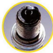
Fouling with dry combustion deposits
