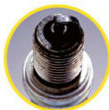
Fouling with non-evaporated fuel
