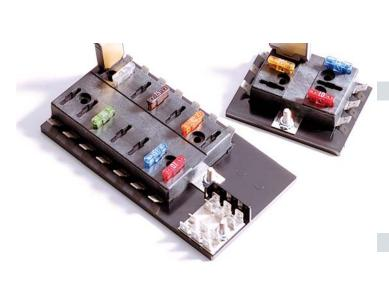
The 15600 ATC<sup>®</sup> fuse panel is a compact, yet rugged, power distribution module. It is available in a single or dual internal buss electrical configuration featuring an optional ground pad terminal strip. The 15600 fuse panel is surface mounted, uses convenient quick-connect terminals, and is recommended as a supplemental power distribution module. It can be used to accompany main PDMs such as the Cooper Bussmann 31000/32000 Series VEC/DVEC, 15710 Series RTA, and the 1540X Series RFRM.
