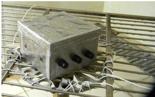
Figure 5. Testing for IP ratings on Eaton's HKP-W-R fuse holders
