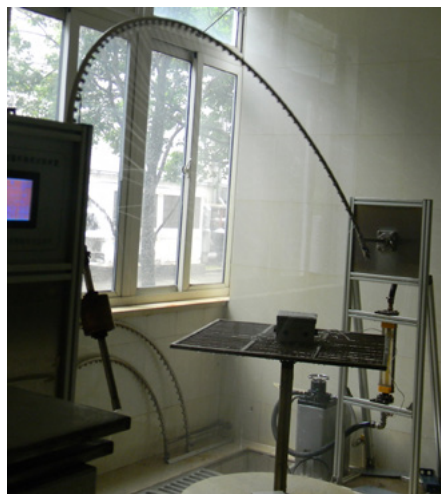
Figure 3. HTB panel mount fuse holders mounted in enclosure and tested to IPx3 conditions at 60 degrees from horizontal
