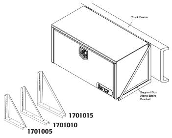
To properly support your Underbody Toolbox, we recommend the use of bottom support mounting brackets. These brackets should be placed so that each end of the toolbox is supported by the full width of the mounting bracket. To prevent rust, touch-up drilled holes with aerosol paint. To prevent water leaks, apply silicone sealant all around each fastener after installation.
