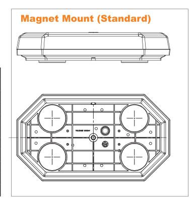
It is not recommended to use magnetically mounted warning devices on vehicles in motion.
