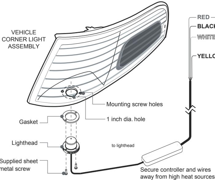
**CAUTION:** Make sure the LED lighthouse does not interfere with the operation of vehicle lights.
