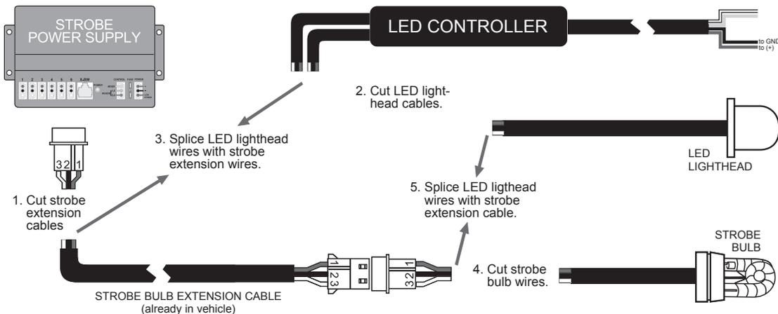
**NOTE:** Make sure that all spliced wires match colors and are well protected from moisture.
