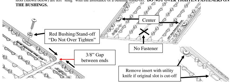
**NOTE:** The screws supplied with this kit are not meant to be used in steel or aluminum, but can be if an 11/64" drill bit is used first to drill a pilot hole. Caution should be used in areas where marker lights and wires have been installed under the trailer deck when installing all fastener.
