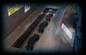
Centric Premium Ceramic Brake Pads are scorched to remove any impurities from the friction material leftover from the manufacturing process. Scorching also preburnishes the pads to greatly accelerate the break-in process.
