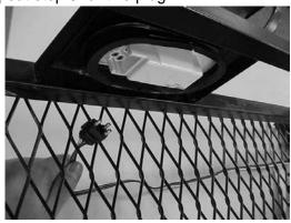
7. Cover wires with black tubing and secure the harness with cable ties to the bottom of the tray.
