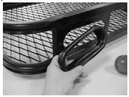
2. Check to make sure the grommet is seated correctly from the inside of the carrier.
