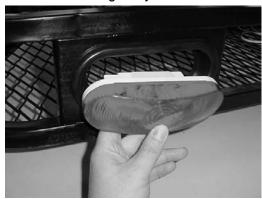
4. Route the 3-way plug with a Yellow wire from under the cargo tray up through the steel grate directly behind the tail lamp housing on driver side of the cargo tray.
