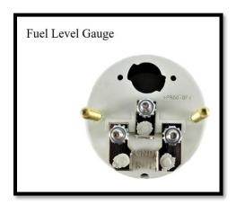
The fuel level gauge will have 4 wires to connect:
