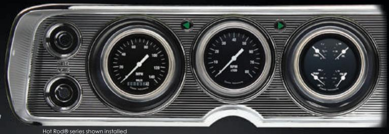
Dash bezel not included. Fuel sending unit not included, fuel gauge is calibrated to stock 0-30 ohms.
