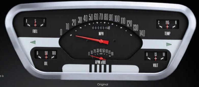
Fuel sending unit not included, fuel gauge is calibrated to stock 75–10 ohms.
