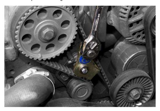
Step 4) While holding the tensioner off of the belt, tighten the adjustment bolt to hold the tensioner in place while you perform your task.
