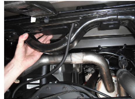
Figure 8.1: Axle Vent Hose Relocation
