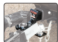
Sway control 17200 shown attached
