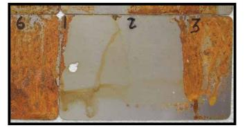
This test was completed after 48 hours. These panels were sprayed regularly with a 5% salt solution. Label 6 is a control with no protection, Label 1 and 2 is the C300, Label 3 is the leading competitor.
