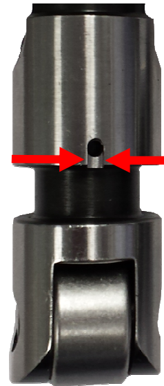
Figure 2: Dart oil galley modification from band to pushrod oil hole
