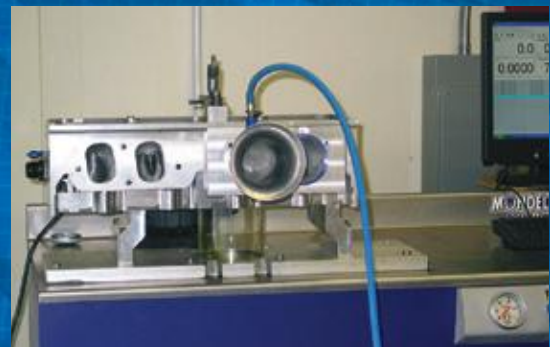
The computer on the wet flow bench captures data about airflow, fuel consumption and air/fuel ratios.
