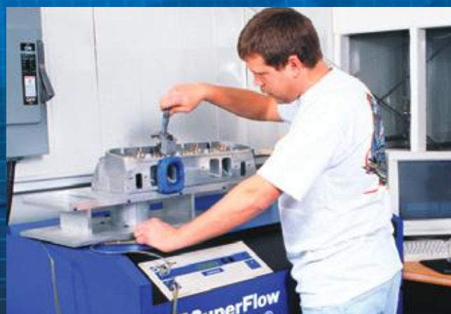
Traditional flow benches are still a useful tool in cylinder head development, but cannot provide any data regarding the fuel handling capabilities of a port or chamber design.
