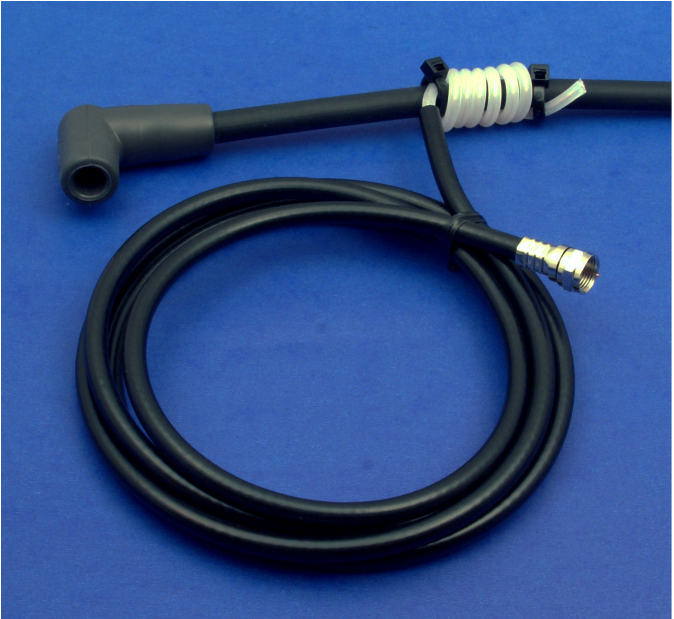
Figure 5 – Capacitive Spark Pickup on Spark Plug Wire
