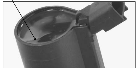
Crack in the epoxy, causes internal shorting
