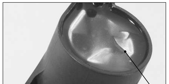
Crack in the epoxy, causes internal shorting
