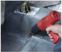
3. After Boom Mat Moldable Noise Barrier is set in proper location, use a heat gun to mold the material to the surface it is being installed on.\*
