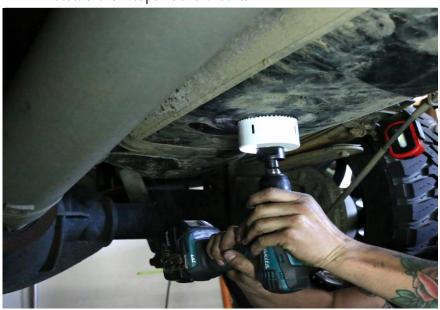
2. With the pilot bit in your hole saw drill through the tank and let the hole saw just scuff the tank.
