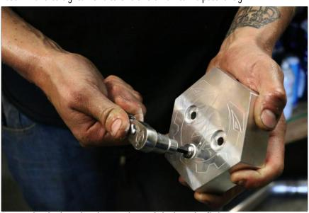
7. Apply thread sealant to the push lock outlet fitting.
