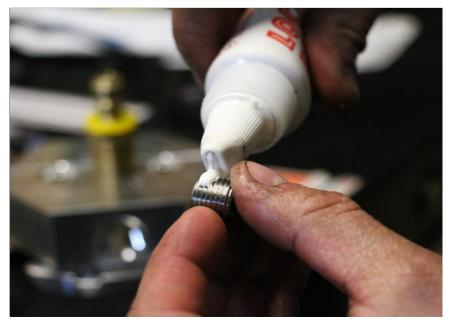
6. Thread the plug into the sump bowl. These are tapered threads we recommend to tighten one to one and a half turns past "snug"
