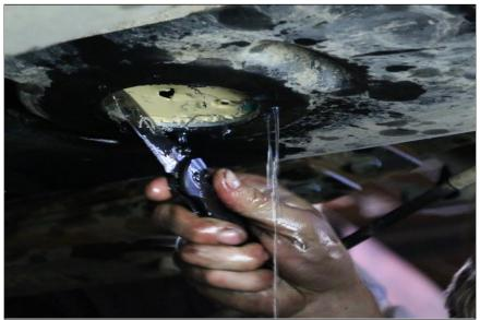
5. Apply a small amount of thread sealant to the 1/4" NPT drain plug.
