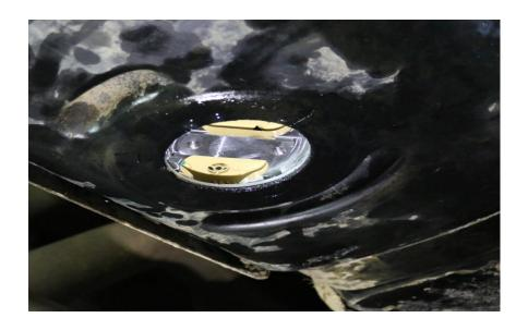
Push sump bowl up into the 3 1/4" hole and thread the two bolts in. Spin the sump in the hole to make sure it is seated. Tighten evenly to 10FT LBS.
