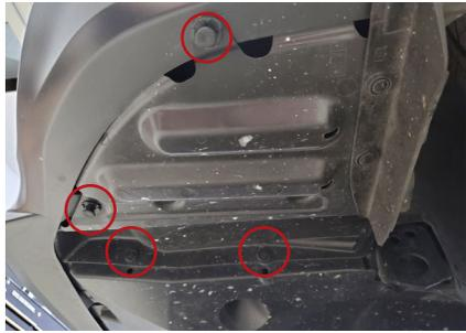
3. Use a plastic trim removal tool to remove the four push rivets on the outer splash guard. Gently pry the splash guard down to gain access to the fog lights. The splash guard will still be connected to the inner fender liner. It should not be necessary to completely remove it unless desired.
