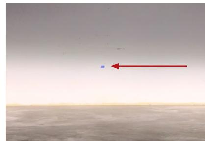
12. Aim your SS3 pods on each side, so that the top of the beam pattern is on the cutoff line mark.
