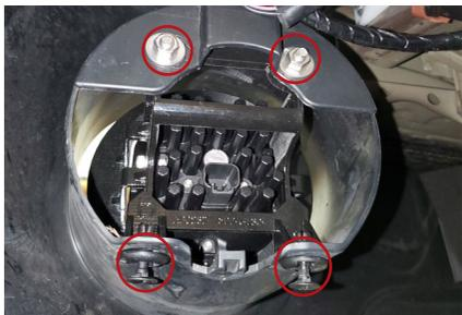
4. Unplug the fog lamp connector. Use a plastic trim removal tool to remove the two plastic push rivets along the bottom of the lamp. Holding the front face of the lamp, use a 10mm socket to remove the two nuts and gently pull the lamp out the front of the bumper opening.
