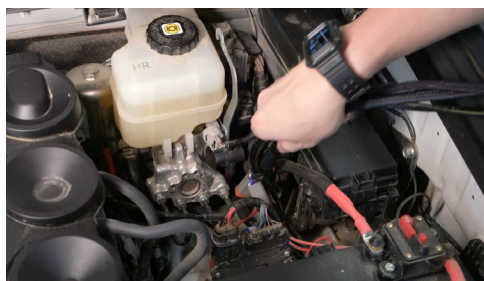
13. Route the connector end of the harness down underneath the vehicle however you see best fit. For this application, we recommend following the wheel well underneath, making sure to avoid any hot or moving parts.
