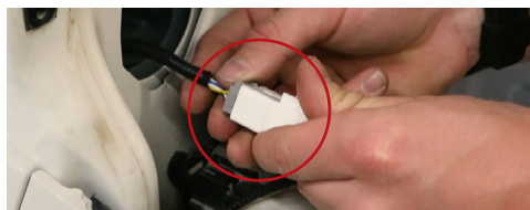
8. Plug the male end of the provided vehicle specific adapter harness into the OEM harness. Then tuck the other end inside the vehicle before reinstalling the taillight.
