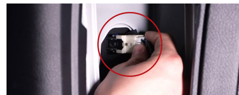
9. Move the taillight back into position and reinstall the two factory nuts. Then plug in the other end of the provided vehicle specific harness into the back of the taillight.
