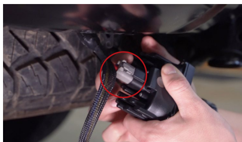
14. Plug the DT connector into the back of the pods and the amp connector into the provided universal harness coming from the taillight D .
