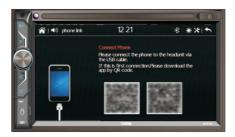
For iOS devices (supported iPhone 5 to iPhone XS), mobile phone linking operation will start automatically without any setting. Mirror linking appeared on the screen.
