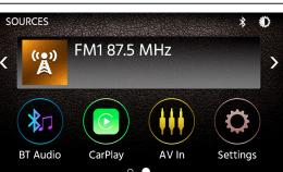
In main menu, press the desired icon to enter the corresponding mode: Radio/USB/CarPlay/ BT Phone/BT Audio/AV In/Settings.
