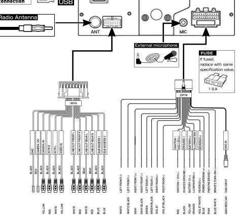
When replacing a fuse, make sure to use the correct type and amperage. Using an incorrect fuse could cause damage. The unit uses (1) 15 amp ATC mini style fuse located on the power connector.
