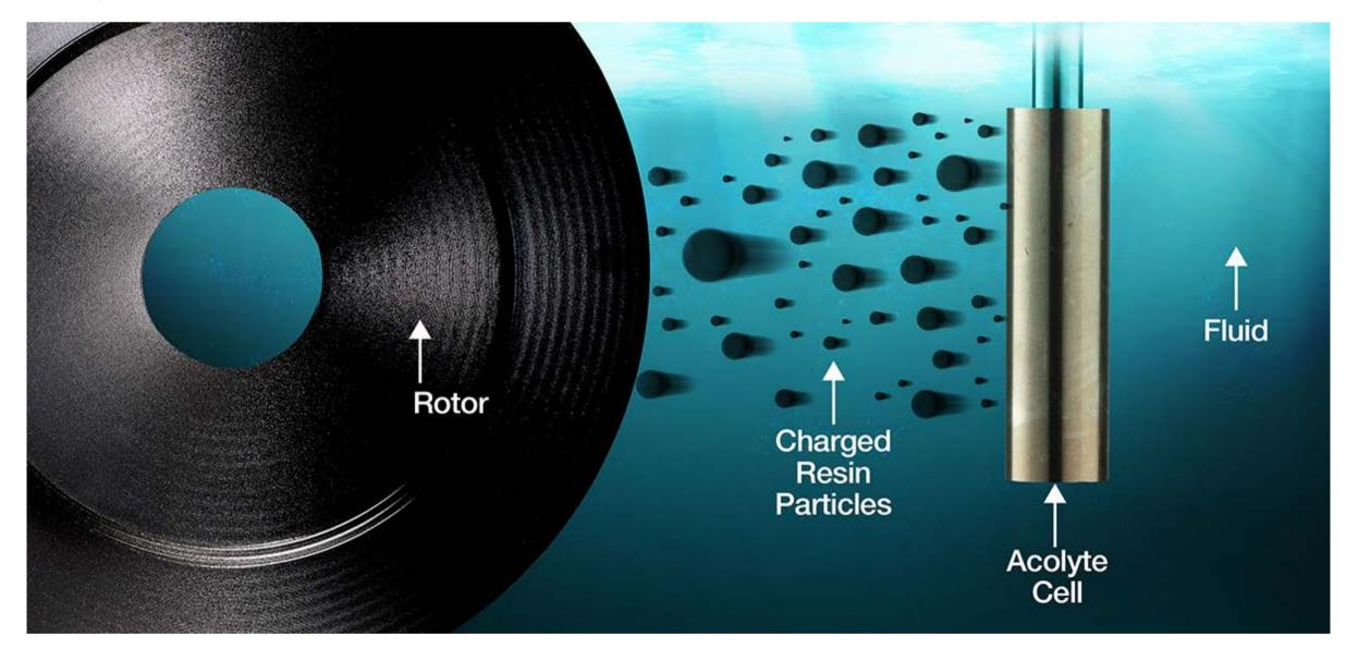
DuraGo Electrophoretic Brake Rotors are thoroughly coated including the inner vanes. Unlike a sprayed on paint, the rotor is fully immersed into a tank and coated by the process of Electrophoretic deposition.
