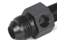
AT100197ERL -8 Male to 1/4 NPT with 1/8 NPT in hex
