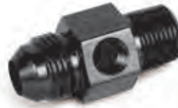
AT100198ERL -8 Male to 3/8 NPT with 1/8 NPT in hex
