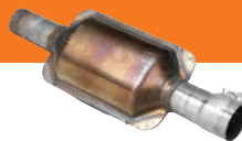
Burned Converter Exhaust temperature too hot.
