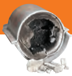
Melted Brick Engine operating too hot.
