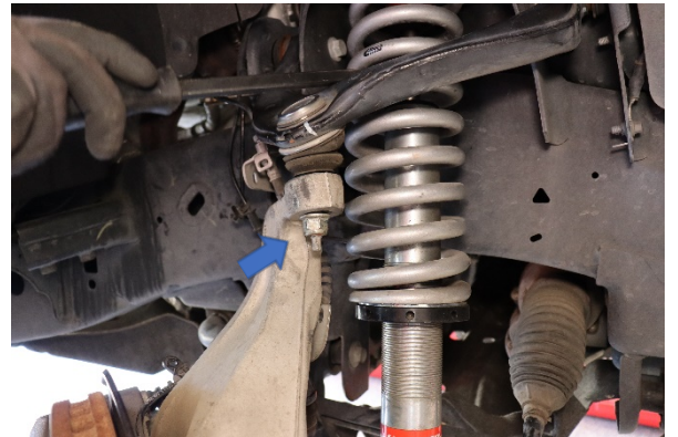
Step 15. Use a pry bar to ease the upper control arm down into the spindle and fasten the nut on the bottom.
