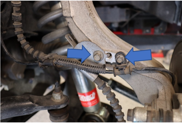
Step 1. Loosen and remove the wheel speed sensor bolt along with the brake hose bracket bolt and set them aside.
