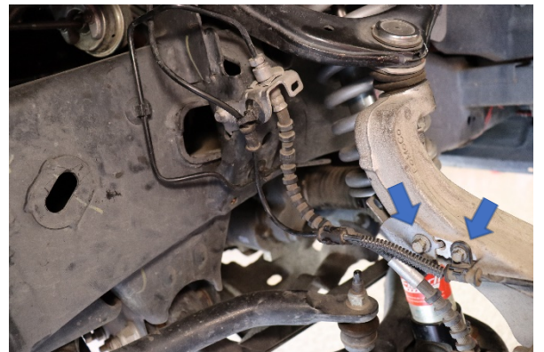
Step 17. Reattach the wheel speed sensor bolt along with the brake hose bracket bolt.
