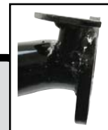
Re-Designed New Level Fit Mufflers and Collector is Centered on Header at 1:00 Position
