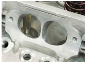
GTV-2 Stage 1 Wedge-Ported Cylinder Head
