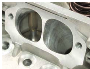
GTV-2 Stage 3 Wedge-Ported Cylinder Head
