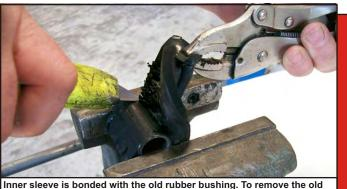
Inner sleeve is bonded with the old rubber bushing. To remove the old rubber bushing from the sleeve, clamp the sleeve in a vice and using a utility knife, slice the bushing longways away from yourself. Clamp the bushing with vicegrips pulling the rubber back and slice as close to the sleeve as possible. Rotate the sleeve in the vice until you get all the way around. Clean as much rubber off the sleeve until smooth.
