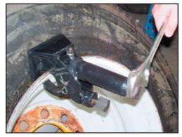
5. Turn bead breaker nut clockwise to engage foot with bead.
