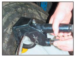
3. Tighten rim clamp jaw until "snug" with hand wrench. Make sure bead breaker teeth and foot are against bead.
