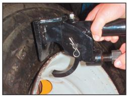
2. Place bead breaker onto the rim with teeth and breaker foot between rim & tire bead.
