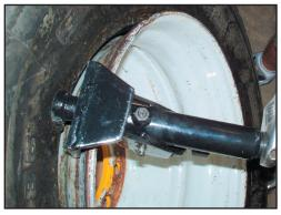
6. Continue to turn clockwise until bead is broken loose from rim. Process may be repeated in 2 to 3 locations on each side of the wheel.
