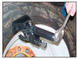
5. Turn bead breaker nut clockwise to engage foot with bead.
