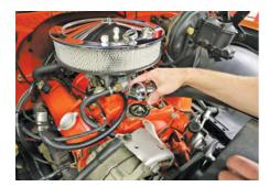
With the block drains still removed, pull the thermostat housing and thermostat from the top of the engine.
