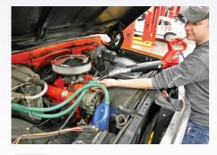
Evans recommends high-volume air for this job, such as a leaf blower. Compressed air can also be used, but it isn't as effective and can cause damage if you're not careful. Blow any remaining coolant out into the container.
