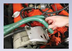
Next task: Remove any residual coolant from the heater core if accessible. Locate the feed and return heater core hoses and disconnect them both from the engine. Stick one in an empty catch container, and if you have an in-line valve anywhere in either line, be sure it's open.
