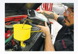
Close up your block drains and petcock, and fill the engine with Evans Waterless Coolant. Burp the system, close up the radiator cap, and run for ten minutes after it hits operating temperature. Let it cool.
