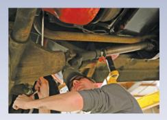
Drain the radiator and the block again, using the petcock and block drains. Save the Prep Fluid, as it's reusable up to three times — but be sure to keep it in a closed container, as it will pull moisture from the air if left out. If you don't get all the Prep out of the system, don't sweat it — it's also waterless and compatible with Evans Waterless Coolant.
