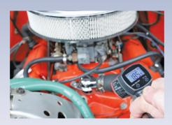
For the Prep Fluid to do its job, it must circulate through the entire cooling system — so you need to get the engine to operating temp, with the thermostat open and the heater running. We used a mini laser pyrometer (Summit Racing p/n G1054) — a handsfree gauge — to verify the truck's thermostat had opened and that all heater hoses were hot. Run for 10 minutes beyond that point, then allow the system to cool.
