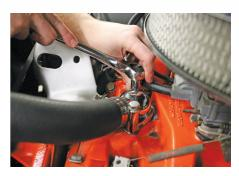
Reinstall the thermostat and housing, the heater core hoses, the block drains and the lower hose (if applicable), and close the radiator petcock.
