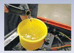
Evans Prep Fluid is specifically designed to pull any remaining moisture from your cooling system. Fill the radiator with Prep, check for leaks, hook up the battery and start the engine. We used Lisle's Spill Free Coolant Funnel (Summit Racing p/n LIL-24680) to burp air out of the system.
