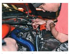
and the old coolant began to rush out. Because it's vacuumed sealed it eventually stopped, but then when we removed the cap it once again began to flow quickly.
