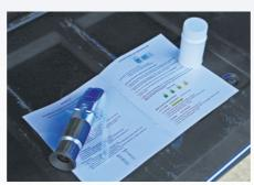
Testing water content is critical—you need less than 3% water for a successful conversion. Evans uses two different methods: a refractometer that uses a Brix scale to measure moisture, and small test strips that come inside the Conversion Kit.
