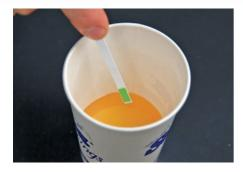
To use Evans test strips, first draw an ounce of coolant from your radiator into a clean container and allow it to cool below 100 degrees. Pull a test strip out of the container and place it in your coolant sample. Move it around for 20 seconds. Then remove the strip and let it sit for two minutes and 20 seconds.
