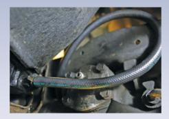
Key to this process is removing as much of the old coolant from the system as possible. Open the radiator cap and the petcock to allow coolant to drain out. To limit the mess that coolant raining on the steering box will cause, stick a two-foot length of 3/8-inch fuel line on the end of the petcock and put the other end into a large bucket. Let it run until it stops.
