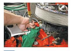
Blow through the block, pushing any remaining water and coolant out of the block drains. If you can't get to the drains or there aren't any, pull the lower radiator hose and place a bucket under it to catch what's in the block. We used high-pressure compressed air, an air nozzle, and a rag. When the block is dry, reinstall the thermostat and housing.
