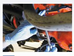
A small-block Chevy has two water-jacket drains — one on each side of the engine just above the oil pan — stopped up with threaded brass plugs. If you can get to them, use a six-point 9/16-inch socket and a ratchet and loosen both to hand-tight, but don't remove them yet. (If you can't get to the drains or can't get them out of the block, don't worry — we'll get to that in a second.)
