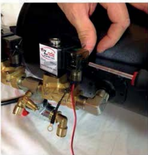
Once wires are connected, put the wiring unit back into it's housing and screw it back on to the solenoid.
