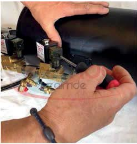
Starting with the left valve assembly (the front), take off the solenoid cap from the intake valve w/ Philips Head (nearest to tank port).
