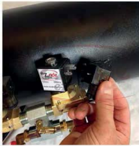
Simply, unscrew and pull the cap off.
