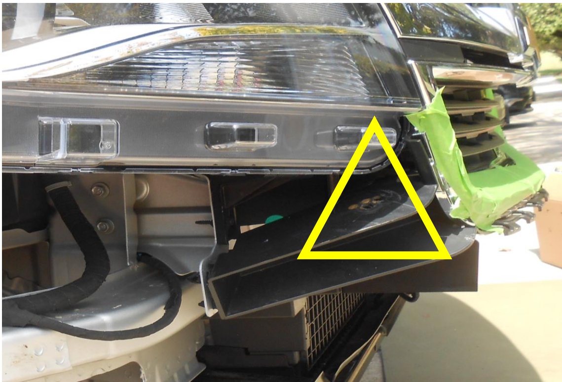
Figure 5d (mount point on plastic grill mount)
