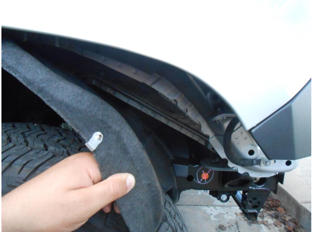
Figure 6a (wheel well liner pull back)
