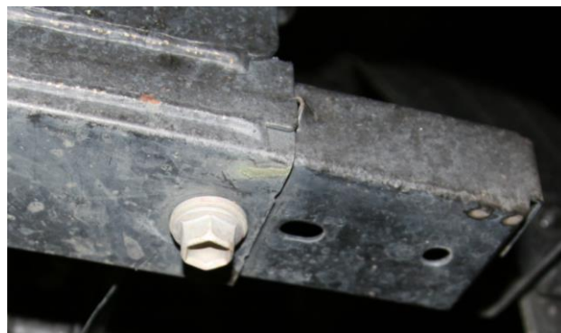
Figure 11 & 12 – Bumper beam extension and tow eye removal
