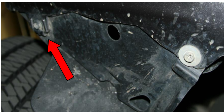
Figure 5 & 6 – OEM bumper cover screw removal
