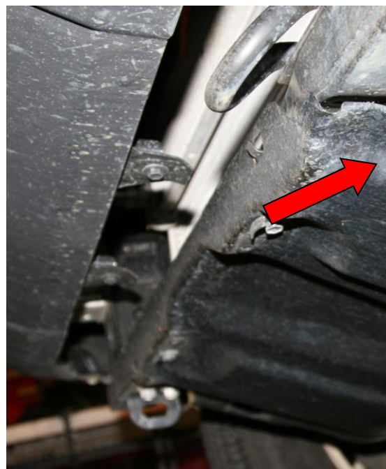
Figure 5 & 6 – OEM bumper cover screw removal
