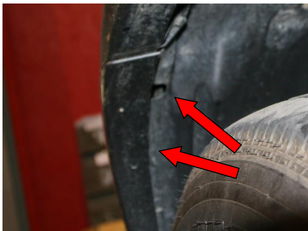
Figure 4 – Fenderwell fastener removal
