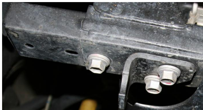
Figure 11 & 12 – Bumper beam extension and tow eye removal
