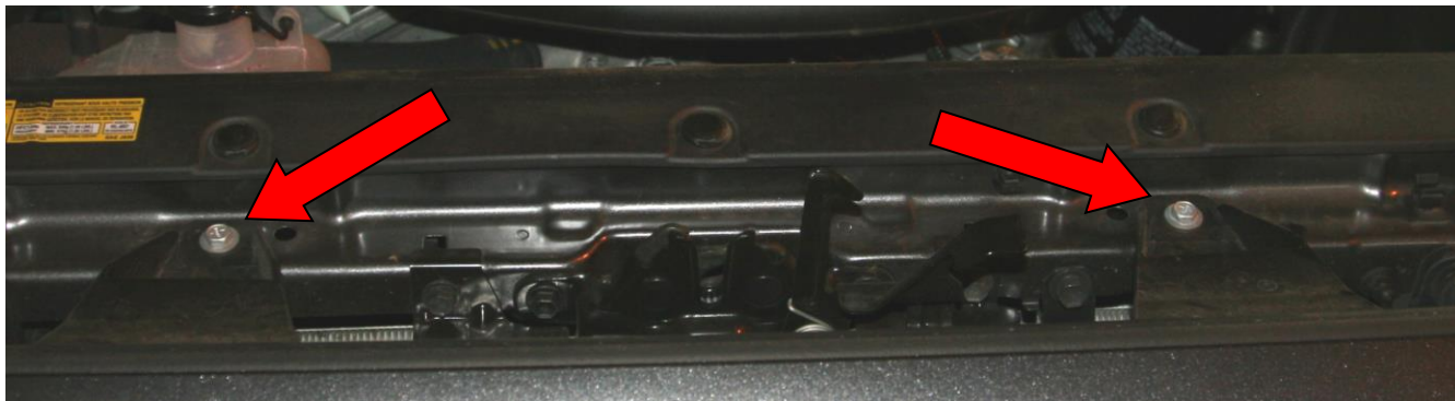
Figure 1 – Upper grill screw removal
