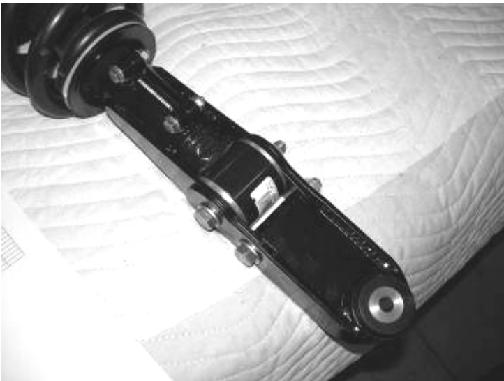
19. Locate the factory upper shock hardware. Install the shock into the factory shock bucket and leave loose. SEE PHOTO BELOW.
