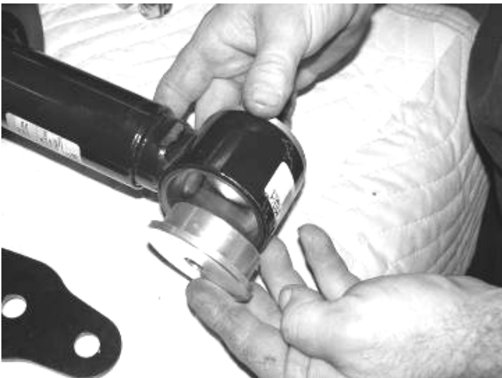
Photo shows installation of FT20342 non-auto ride aluminum bushings
