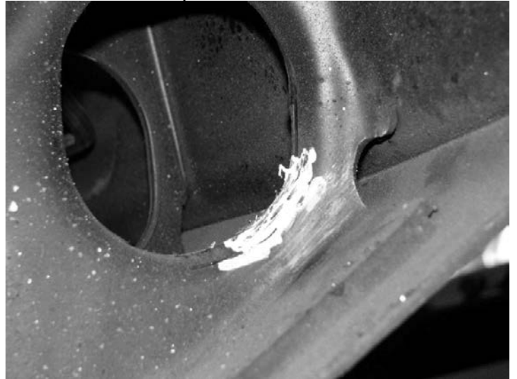
40. Locate the factory crossmember the torsion bar runs through. This cross member will need a small amount of clearance added to it. At the intersection of the frame and the crossmember, grind a 2" Radius 1/4" deep. SEE PHOTO BELOW
